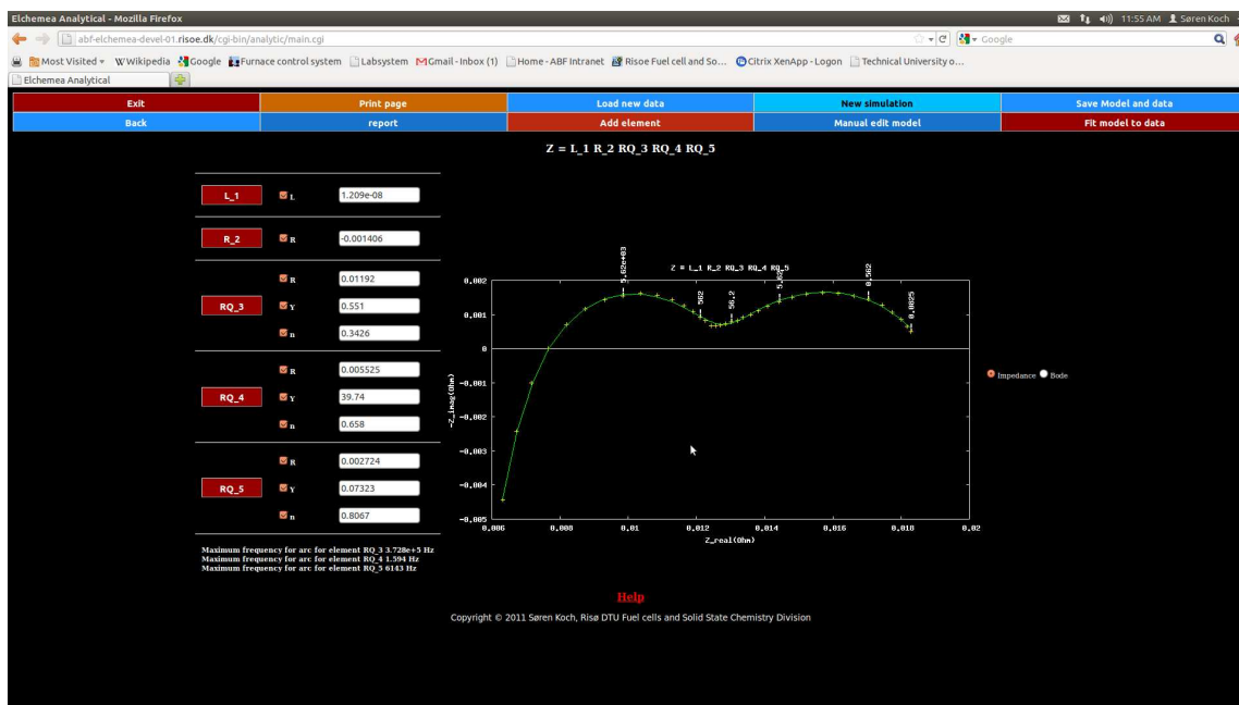
Figure 3.7: Example result of a fit of a model to an actually measured impedance spectrum.
